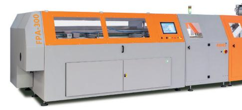
FPA-300 - Fully automatic pocket spring assembler
